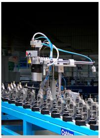
alkitronic® PV-F operating in a preassembly and final assembly workstation. Remote controlled continuous tightening in semi-automatic operation.
